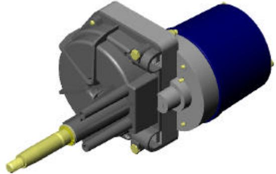
Tilt Shaft with Rudder Feed Back
