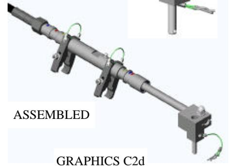
C2e. Assemble Connection Kit & Second Steering Cable to Steering Cylinder
