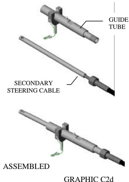
C2e. Assemble Connection Kit & Second Steering Cable to Steering Cylinder
