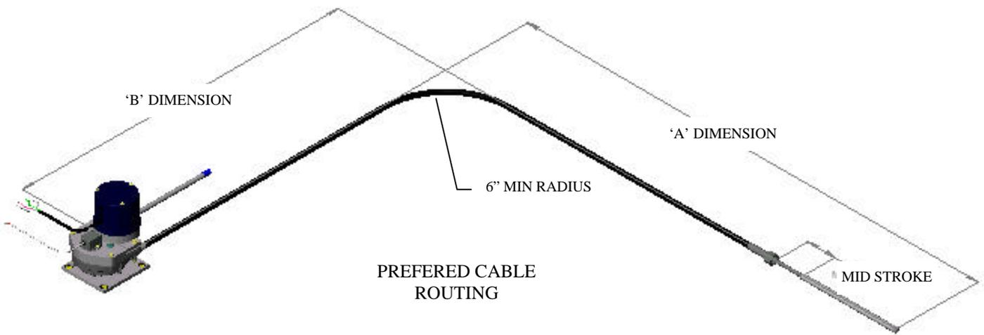
EXAMPLE OF STEERING CABLE LENGTH CALCULATION:
