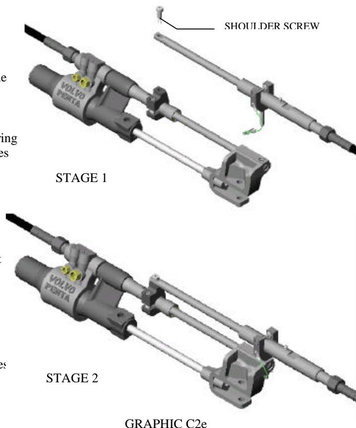
C2f. Axially Position Drive Collar and Tighten Clamp Screw
